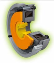
The tacho brake has a fixed distance ring as well as a centering recess and three tapped holes on the rear side of the coil carrier. The centering recess is centered with the outer diameter of the distance ring.
